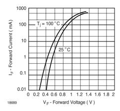
Figure 1. Forward Current vs. Forward Voltage
