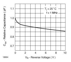
Figure 4. Relative Capacitance vs. Reverse Voltage
