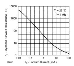
Figure 2. Dynamic Forward Resistance vs. Forward Current
